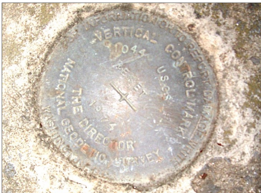
NATIONAL GEODETIC SURVEY BENCHMARK on the step outside of Salem’s vestibule. The benchmark indicates an elevation of 1044 feet above sea level.
